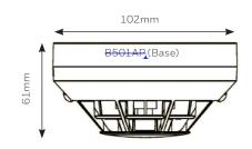
The HM-PTSE conforms to EN54-7, a 58°C fixed temperature and rate of rise thermal assistance conforming to EN54-5. The thermal detection function combines thermistor technology with a software corrected linear temperature response. In areas where the normal daytime activities may potentially create unwanted alarms, the detector can be programmed to operate in a "heat only" mode, automatically reverting to full photo-thermal operation during unoccupied periods.
